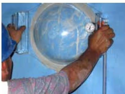
Vacuum testing using a vacuum bell and electrical vacuum pump for testing of details. After treating the seam edges with soap solution, the vacuum bell is firmly pressed over the area to be tested and the vacuum applied. Any leaks are clearly seen by bubbling of the soap solution under vacuum.
