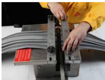
Butt-jointing of waterbars by heat welding using the semi-automatic welding equipment SG 320L.
