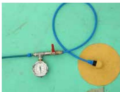
Vacuum testing of compartments of a double layer membrane system using vacuum pump. During the testing the vacuum should not drop less than 20% in 10 minutes to be completely watertight.
