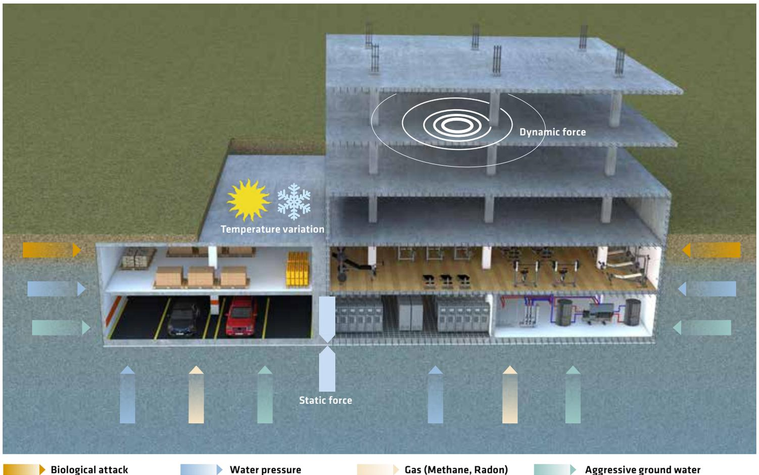
Yellow arrow: Biological attack      Blue arrow: Water pressure      Orange arrow: Gas (Methane, Radon)      Green arrow: Aggressive ground water
