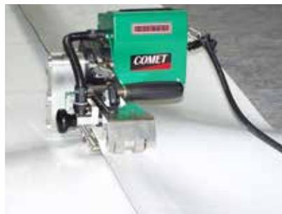
Automatic hot air, or heating wedge welding machine with clamped pressure roller, welding temperature, pressure force of rollers and speed are adjustable. Suitable for single seam and double seam welding with air pressure channels between seams.
